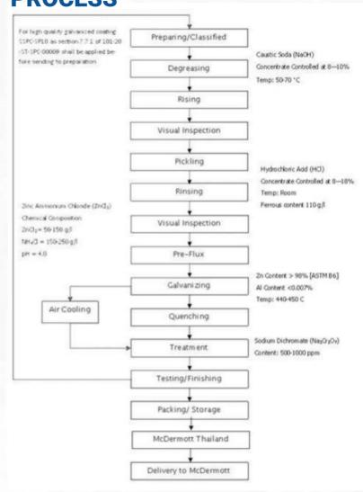
It involves cleaning steel and immersing it in molten zinc to obtain a coating.
