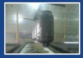
3. Rinsing/Visual Inspection The caustic cleaning solution is rinsed off.
