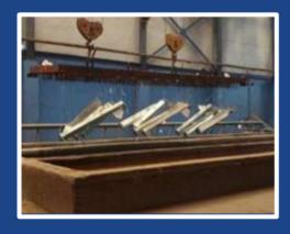
6. Pre-Flux A flux, often zinc ammonium chloride is applied to the steel to inhibit oxidation of the cleaned surface upon exposure to air. The flux is allowed to dry on the steel and aids in the process of the liquid zinc wetting and adhering to the steel.
