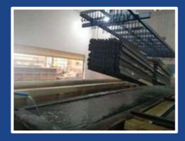
4. Pickling Hydrochloric Acid (HCL) Concentrate Control at 5-18% The Steel is pickle in an acidic solution to remove mill scale and oxide.
