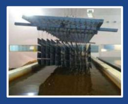
5. Rinsing/ Visual Inspection The next and final bath before the actual zinc dip is a low-pH zinc ammonium chloride mixture which acts as a fluxing agent. It also contains a chlorine salt that encapsulates the metal and pre-vents it from oxidizing again
