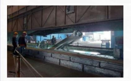
8. Quenching: Cooling When the steel is removed from the galvanizing kettle. The quench tank contains mostly water help cool it down before the final cleaning process.
