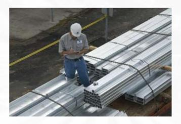
The steel is then moved outside and placed on poles for millage tests. These tests verify that the process was successful and that the zinc coating is the proper thickness. Different applications for the steel can call for different coating thickness.
