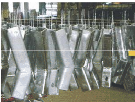
High Silicon Reactive Steel results in extra zinc pick-up and causes a dull and brittle grey coating.
